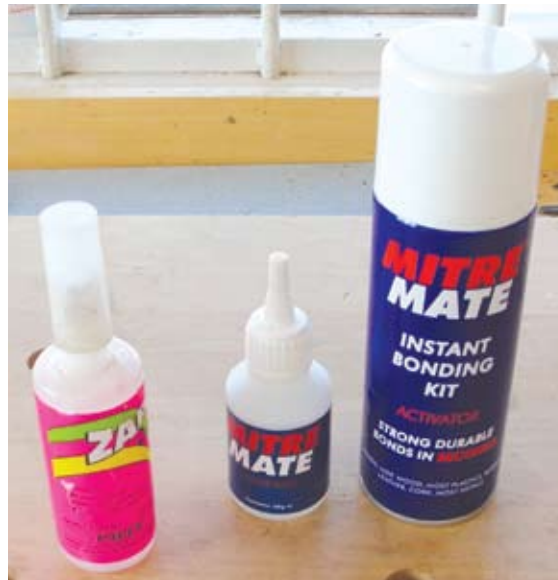
These three super glues work with accelerators to make them worthy of the workshop glue adhesives arsenal
