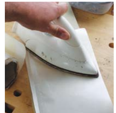
Hot-setting glue film is useful for small veneering jobs
