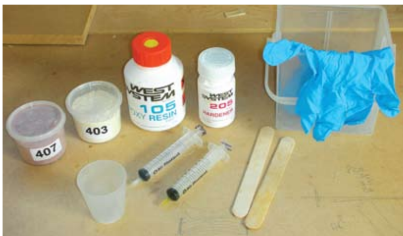
Epoxy resin has to be mixed very carefully but the result is a really strong joint with no glue creep
