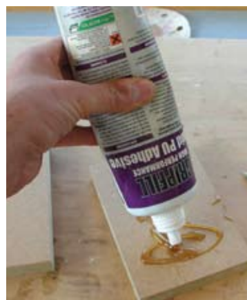
Applying polyurethane adhesive
