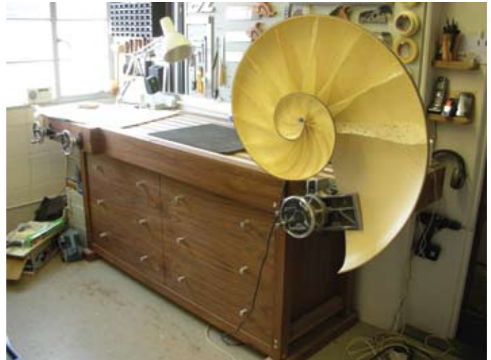
19 The pattern maker's vice allows me to work on some pretty unusual shapes...
