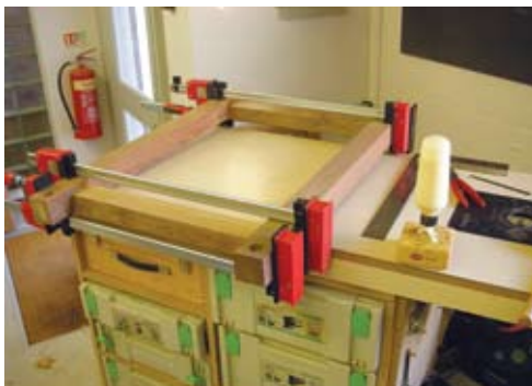
3 The end leg sections were glued up as complete components after the bolt holes had been drilled
