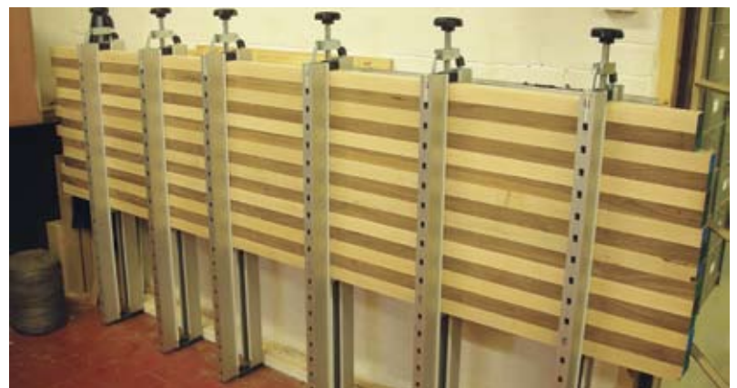
5 The Shepach Plano is designed for jobs such as these but requires the same amount of free space at one end to slide the work top into the clamping frame
