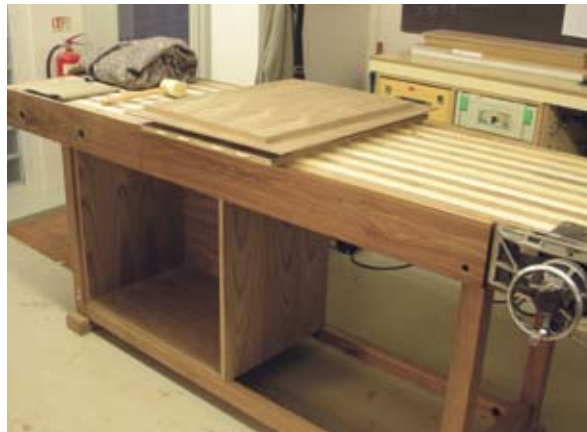
15 The cupboards are fixed in place and, with the back boards fitted, give the necessary bracing to the base frame
