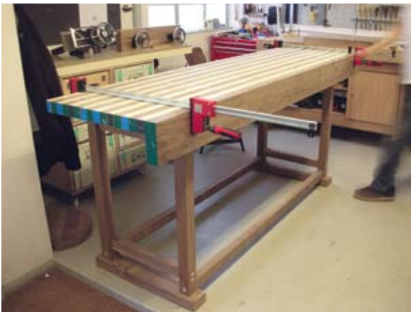
9 The back rail in place on the worktop...
