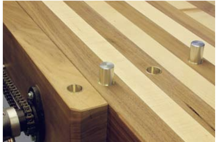
17 Aluminium bench dogs were machined at the same time as the bolt head caps used on the base frame
