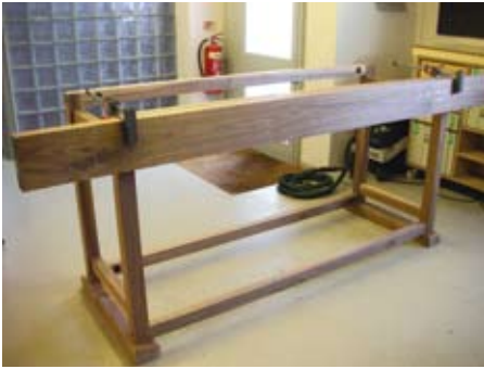
6 The front and back rails were machined well over length and positioned on the frame for marking out of vices and bench dogs along the back edge
