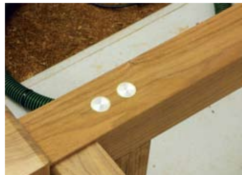
4 Aluminium bolt caps were machined in-house to fit into brass bezels to conceal the bolt heads
