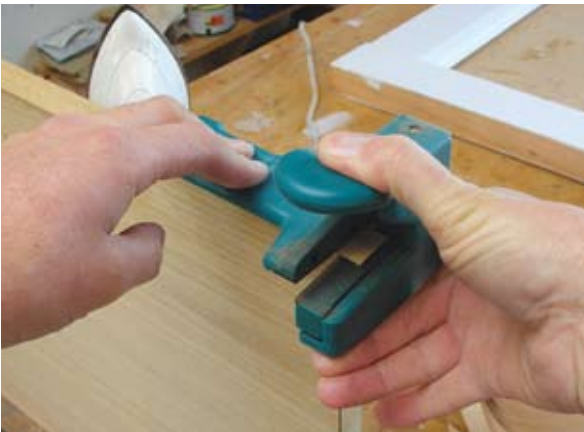
14 End trimmers are a useful investment if you have multiple components to prepare
