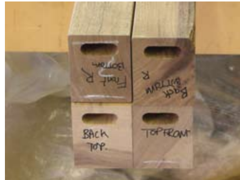
2 Dominoes are the perfect loose tenon and were used throughout the frame with bolts to connect all the components
