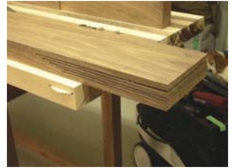
8 ... a series of cuts into the end were later shaped into the taper required for the pattern maker's vice
