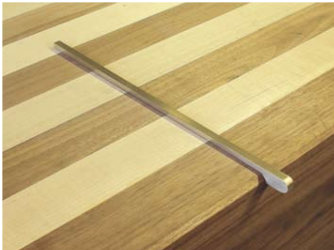
18 Along with the rear bench dogs, a brass bar is used to secure a sacrificial MDF top for work likely to damage the surface
