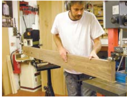
7 The front rail required some elaborate shaping which was started on the bandsaw...
