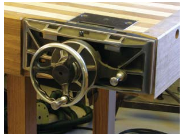
11 Final shaping of the front rail to accept the pattern maker's vice. Similar shaping was required on the end rail which was bolted through slots onto the worktop. The twin screw vice on the other hand was relatively straightforward to fit
