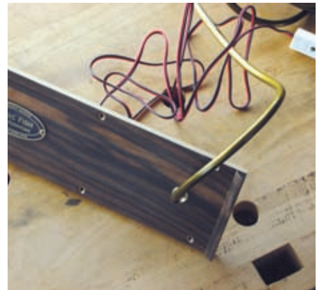
Detail showing how the cable passes through the rear panel
