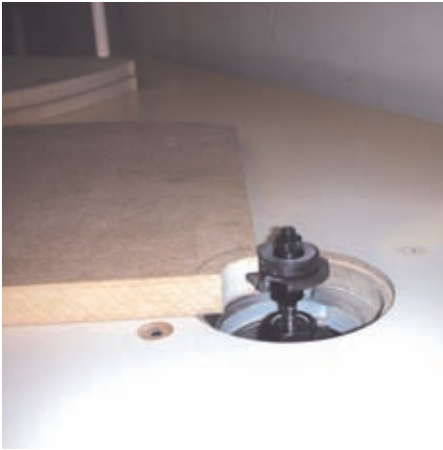
1.1 Routing the slots for the loose tongue in the MDF carcass floors
