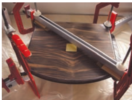
1.8 The setup for clamping the ferrules in place
