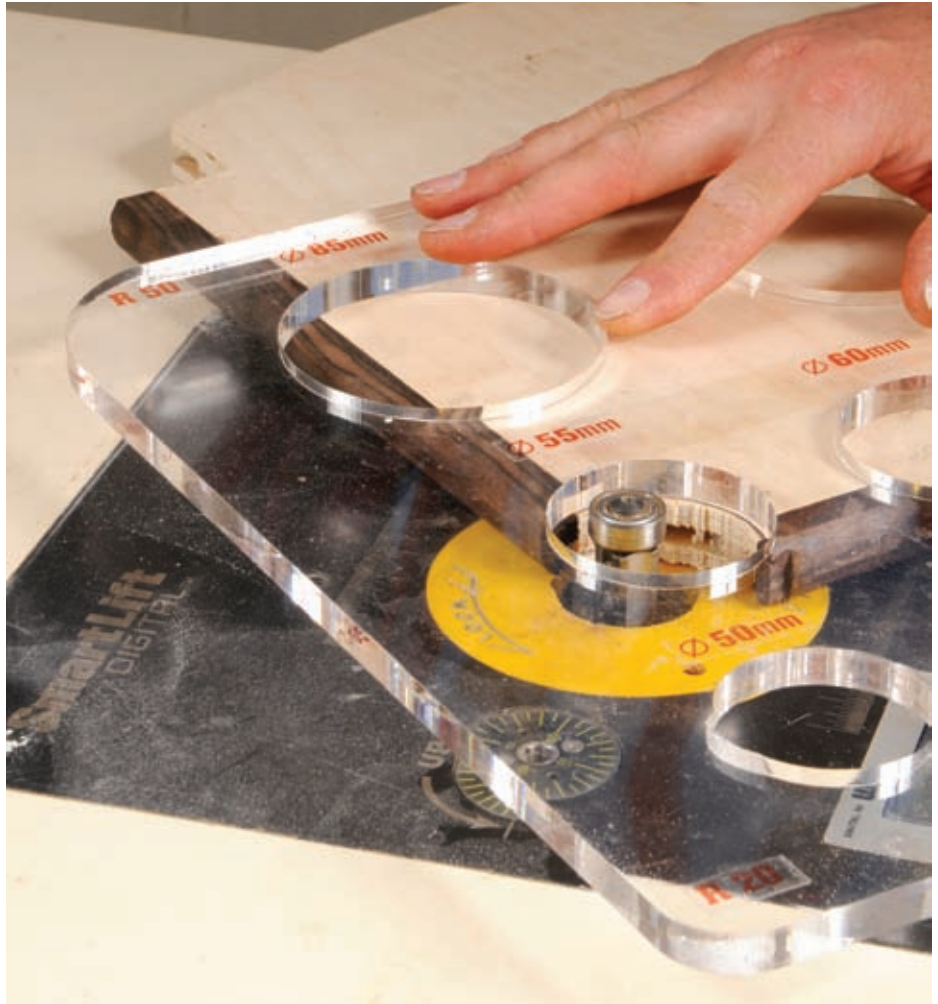
1.3 Use of an acrylic circle-cutting template ensures most of the waste is removed
