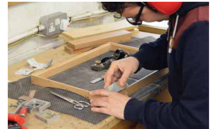
Glue blocks and spacers are cut in advance to ensure the glue-up runs smoothly
