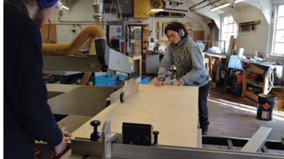
Ripping up a plywood sheet to make the tray base
