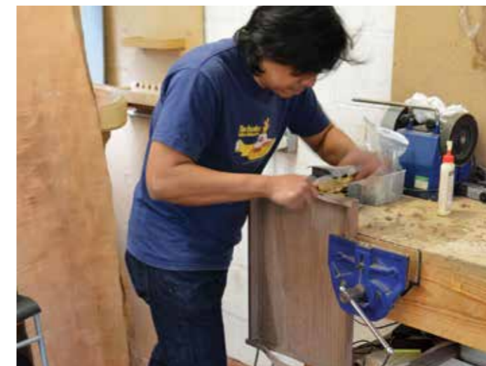
Shaving the handle to fit the frame
