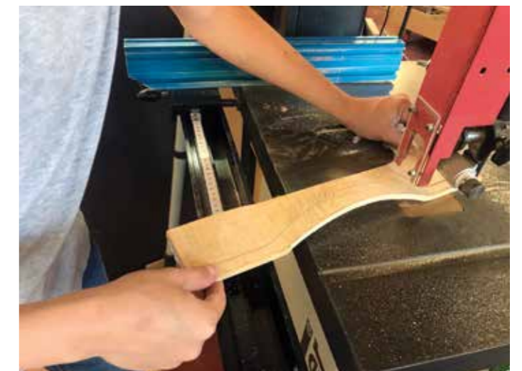
Roughing out the shape of the handle on the bandsaw
