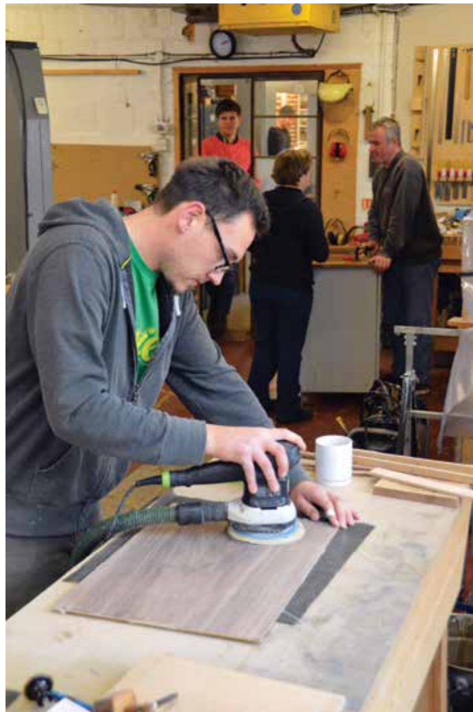
Working through the grits with a random orbital sander
