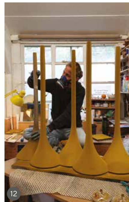
7 The turned brass fit, which will be attached later 8 Progress so far, all bonded together ready for the next stage 9 The deep cone shape in each leg component 10 The tops of the cones coated with metallised paint which is being rubbed back 11 The brass effect starts to appear as if by magic 12 Now for the legs – a respirator is essential because of the metal dust generated
