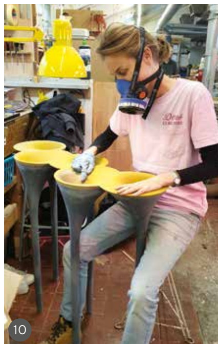
7 The turned brass fit, which will be attached later 8 Progress so far, all bonded together ready for the next stage 9 The deep cone shape in each leg component 10 The tops of the cones coated with metallised paint which is being rubbed back 11 The brass effect starts to appear as if by magic 12 Now for the legs – a respirator is essential because of the metal dust generated
